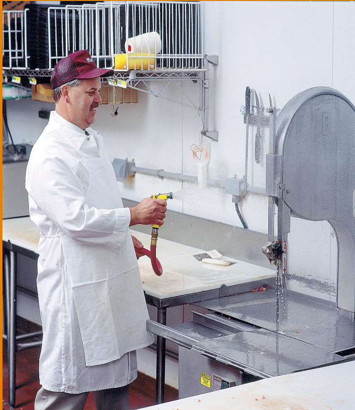
Cleaning fixed equipment
