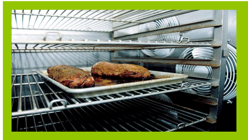
Internal view of rapid chill system
