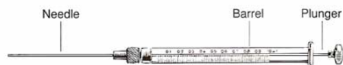
Figure 2-11 Hamilton syringe with a volume of 1 \mu\text{L} and graduations of 0.01 \mu\text{L} on the glass barrel. [Hamilton Co., Reno, NV.]
