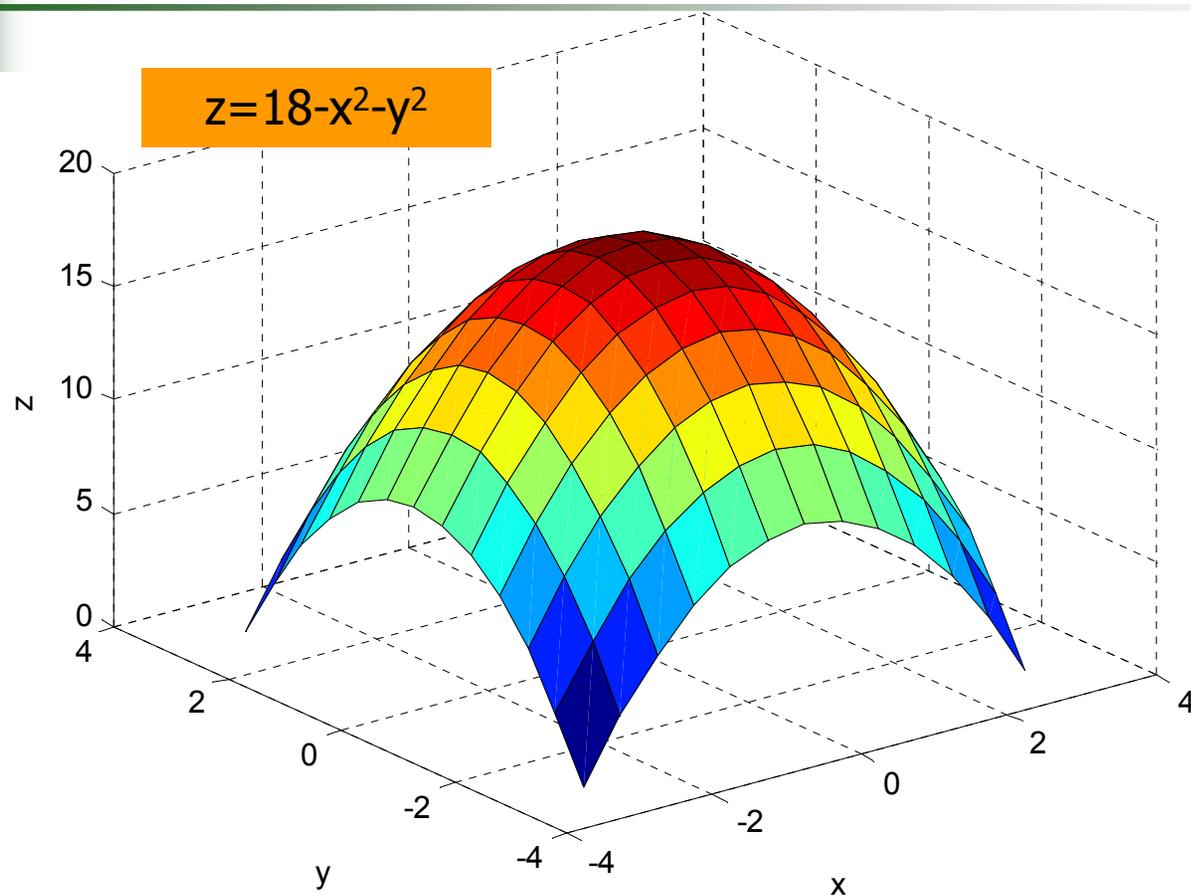
the double integral  $\iint z dx dy$  can be interpreted as the volume under the surface  $z = f(x,y)$
