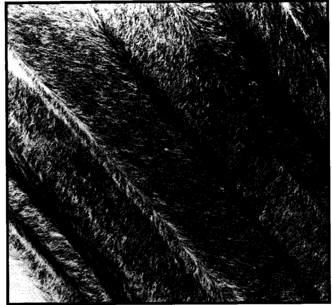
Fig.1.23 Polyamellate structure of a parenchyma cell wall, Phyllostachys pubescens (Syn. Ph. edulis ) 19/000 X. (Courtesy of W.Liese. 1998).
