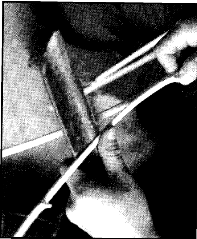
Fig.6.14 The low shear strength of bamboo is an advantage for some purposes, for example in the manufacturing of bamboo strips for weaving baskets and many other articles.
